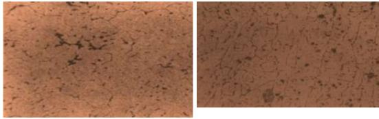
Plate 4.1: Microstructure of Al-Si-Fe matrix Plate 4.2: Microstructure of 18wt% of CSA reinforced Al-Si-Fe composite at 95 °C and at a holding time of 120 mins.
