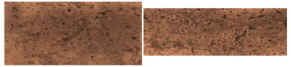
Plate 4.3: Microstructure of 18wt% of CSA reinforced Al-Si-Fe composite at 250°C and at a holding time of 120mins.
