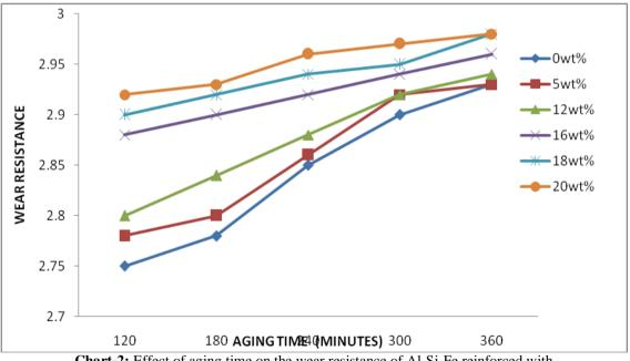
**Chart-2:** Effect of aging time on the wear resistance of Al-Si-Fe reinforced with varying percentage of CSA at 250°C.
