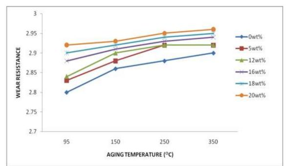
**Chart-1:** Effect of aging temperature on the wear resistance of Al-Si-Fe reinforced with varying percentage of CSA at a holding time of 300mins.
